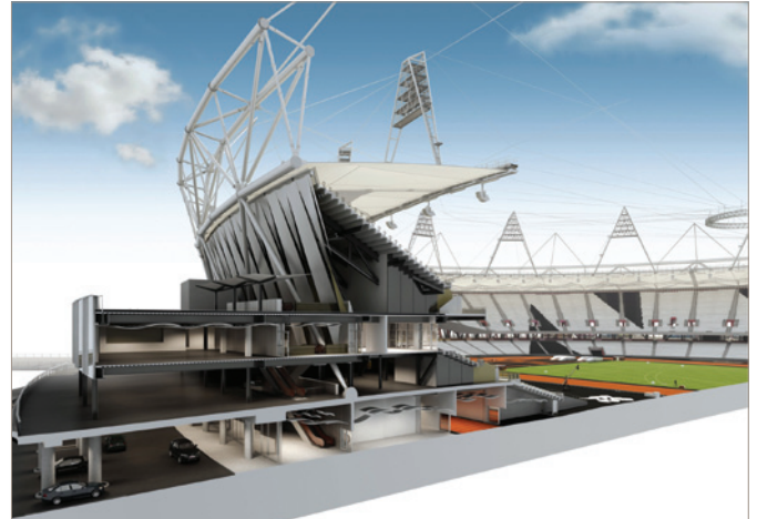
Figure 3. Section through west stand and pavilion showing permanent accommodation areas under temporary seating tier
